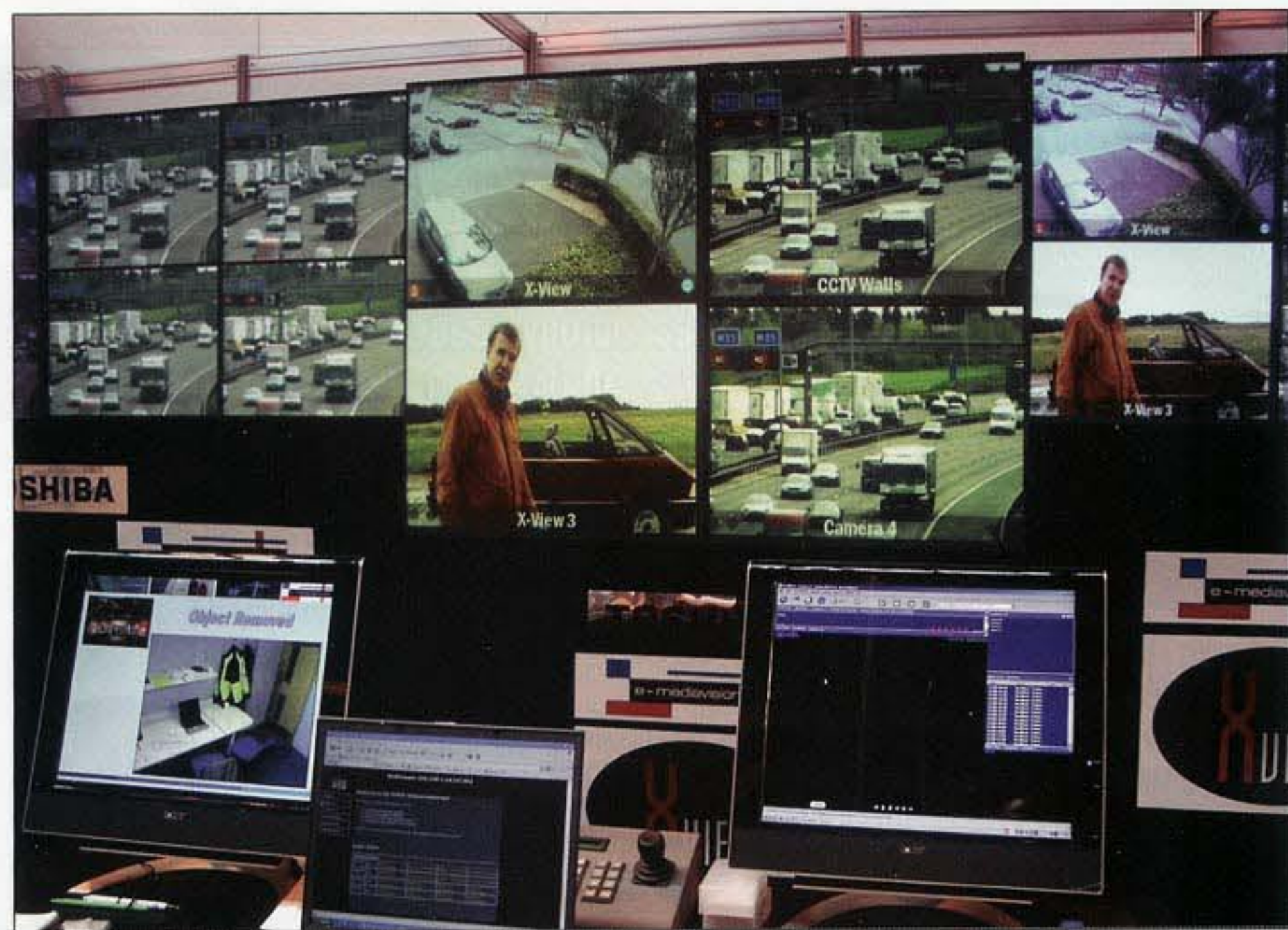
Today's best display processors give operators more immediate access to the most critical information needed at any time. Shown here is e-mediavision.com's X-View command wall system, which enables the monitoring of multi-site systems and the centralization of engineering resources on a 24/7 basis.
