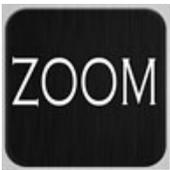
The Zoom button allows the user to draw a rectangle selection on the background, once drawn, the background will zoom up to fill the screen with the selected area of interest. Using this Zoom tool (full screen zoom) will fill the screen with the zoomed up image. The zoom tool in the tool bar only zooms up inside the tool area.
