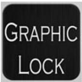
The Graphic Lock button is used to freeze any placed graphics that would normally be movable, such as a Circle, by using the Graphic Lock and freezing the annotations in place you can then use other tools to draw over the placed graphics. Note that the graphics will be locked until you unlock them by clicking once more on the Graphic Lock button to deactivate it.
