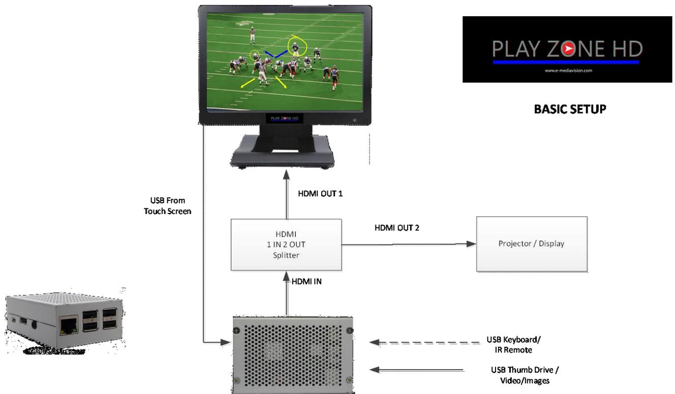
1. Connect the USB from the touch screen to one of the USB ports on the EzPz1
