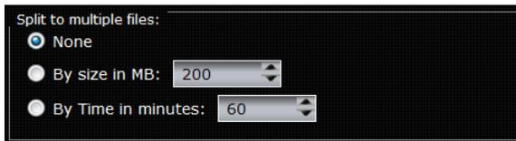
EMV-HDR provides an auto file split functions, which allows long record sessions to be recorded as segmented video clips (either by file size or recording time), as soon as a clip is recorded this can be worked upon, allowing easy and fast after event distribution of video content.
